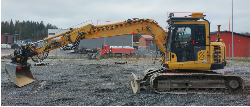
Figure 9: The excavator used in the data collection phase. In the picture, the cabin (1.), boom (2.), arm (3.), and bucket (4.) are highlighted with red boxes [3].
