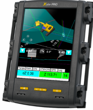
Figure 6: Xsite ® PRO 3D system that is installed in the excavator cabin [31].
