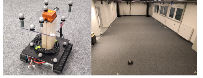
Fig. 2. (left) Differential drive robot. On top of the transparent plastic platform, the IMU and the infrared markers for the Vicon tracking system can be seen. (right) Differential drive robot in the Holodeck laboratory with Vicon cameras on the ceiling.
