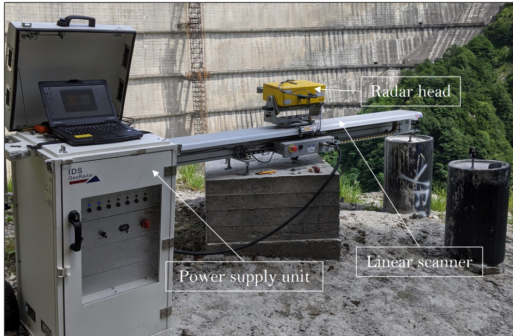
Figure 2.2: Three main components of a GB-SAR system: the radar head, the linear scanner and the power supply unit.
