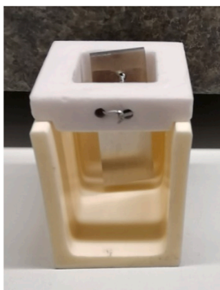
Fig. 1. Cut alumina crucible with a sample fixed to an alumina holder by Mo-wires.
