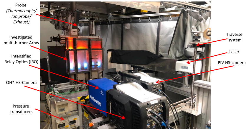
Fig. 1. Photograph of the experimental setup including an optical measurement techniques employed in the investigations.
