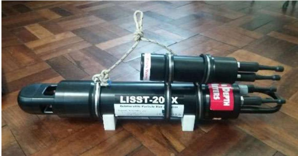
Figure 27 – LISST-200x with the battery attached.
