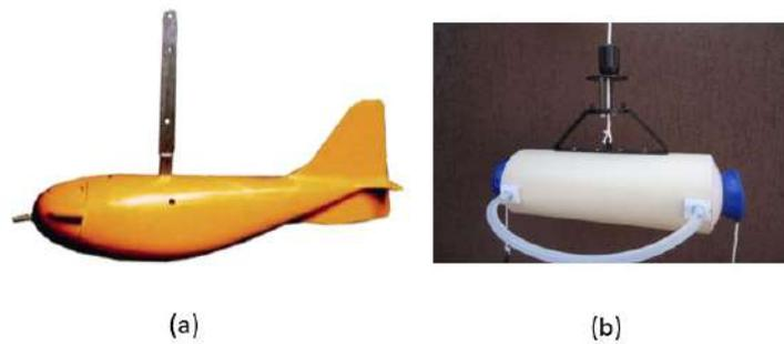
Figure 28 – Water Sampler Devices (a) USD-49 and (b) Van Dorne.
