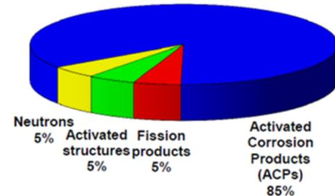
Corrosion products generates gamma radiation fields
