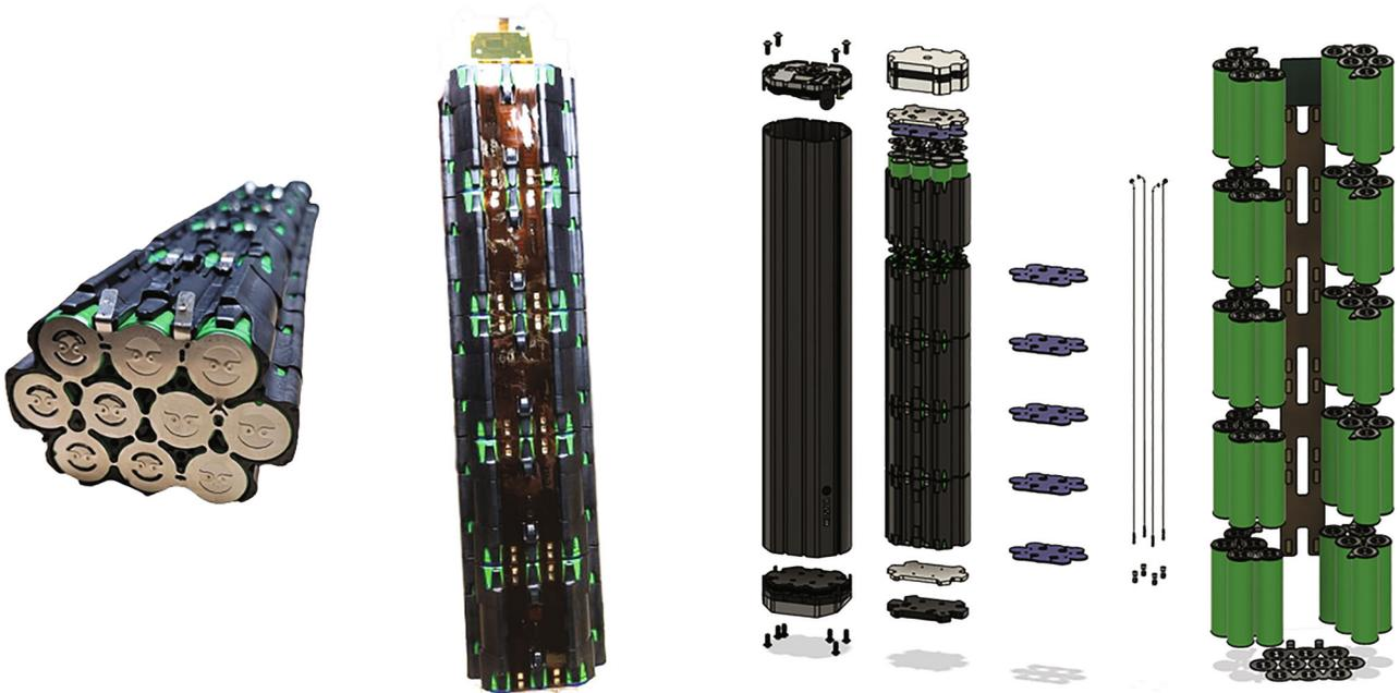
FIGURE 7: Photographs of the original reference system built out of 18650 cylindrical cells and CAD images.
