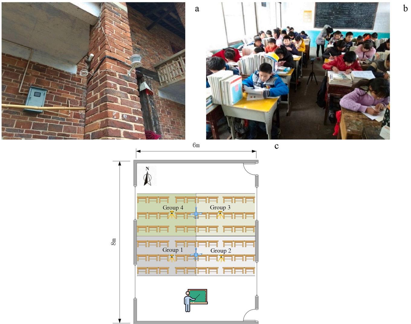
Fig. 1. Physical measurement of (a) outdoor thermal environment, (b) indoor thermal environment and (c) the classroom layout.
