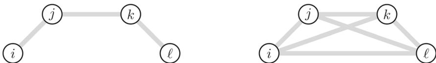
**Fig. 4** Sketch of united-atom butane: On the left-hand side, the molecule with the particles  $i, j, k$  and  $\ell$  is shown including the bonds between atoms. On the right-hand side, the distances between the particles  $i, j, k$  and  $\ell$  used by the discrete gradient are given
