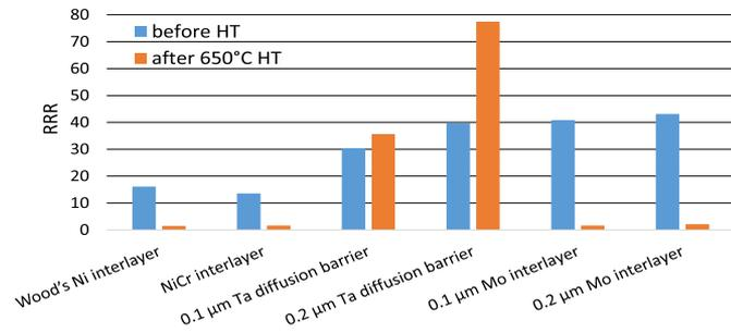
Fig. 4. RRR of Cu coatings before and after the 650 °C-50 h HT.
