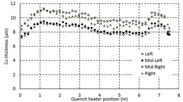
Fig. 3. Typical Cu coating thickness distribution on the four circuits of an MQXFB quench heater.
