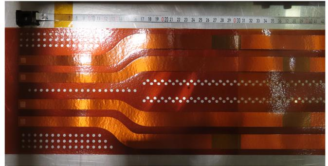
Fig. 1. MQXFB quench heater terminal with coverlay.
