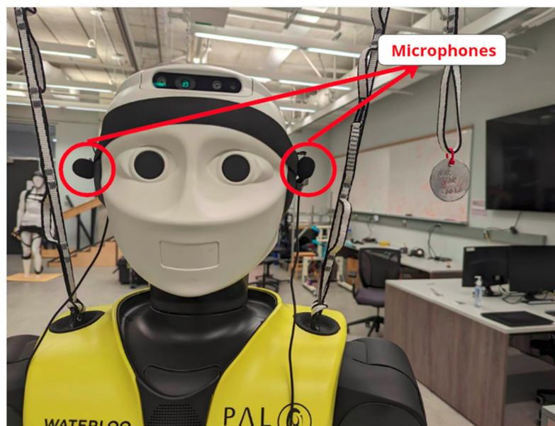
Fig 20. Microphone setup on REEM-C.
