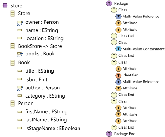
(a) first example metamodel (b) extracted token sequence
