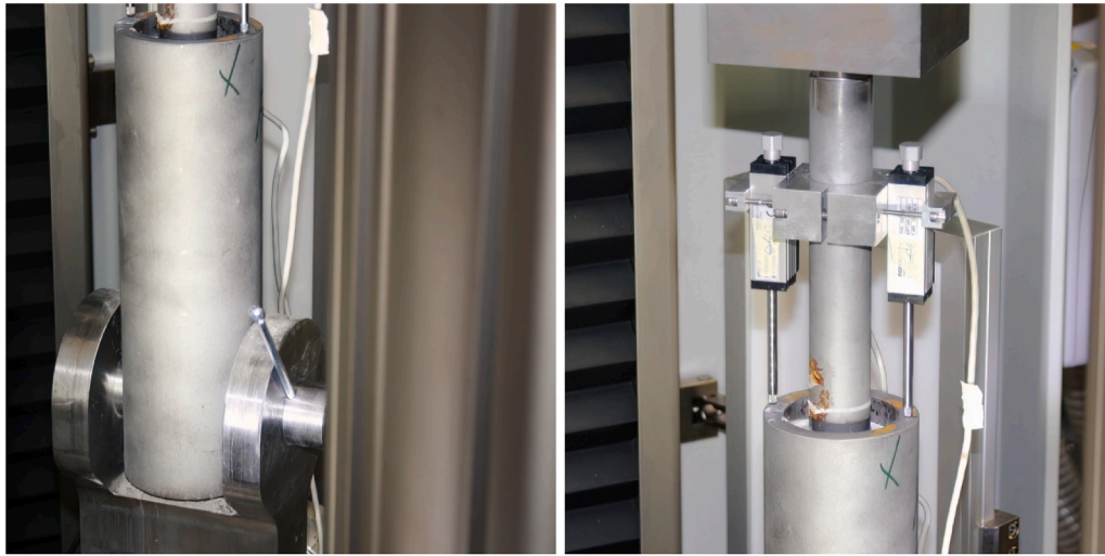
Fig. 6. (left) Hinge at the bottom of the sample, (right) the pair of LVDT measuring the relative displacement.
