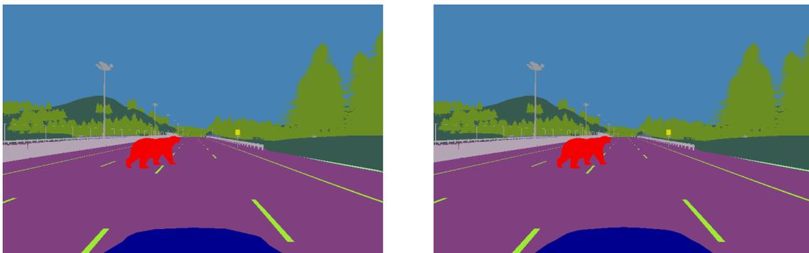
Figure A.3: Comparison between Frame 7235 and 7236 show the misalignment in the engine hood. This resulted in voxels appearing in the prediction voxel grid with high anomaly scores that originate from the predictions on the engine hood.
