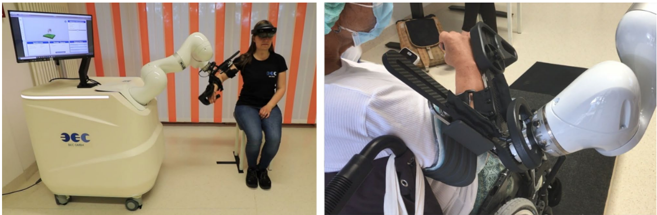
Fig. 1 Left: subject using the RobExReha system with the HoloLens for the gaming application. Right: arm-robot interface used by a patient during the therapy with the RobExReha system
