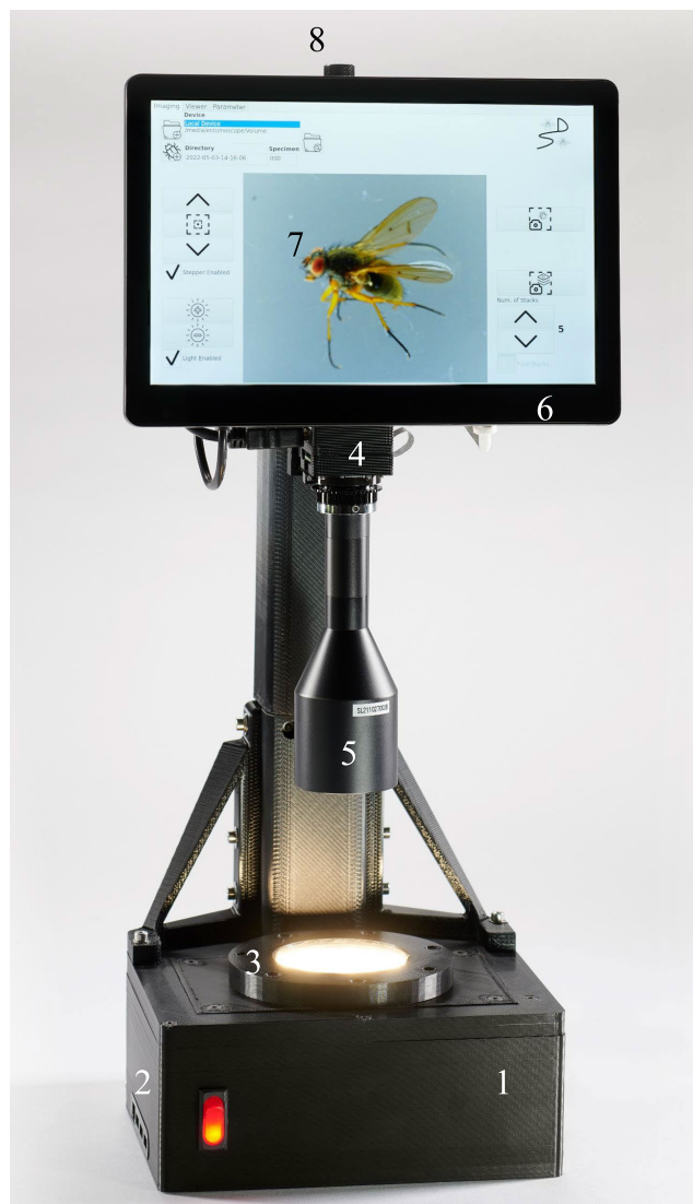
FIGURE 2. The standalone Entomoscope, with (1) base, (2) USB and network hub, (3) lighting, (4) 12 MP camera with (5) telecentric lens, (6) 10" HD touchscreen, (7) Graphical User Interface, and (8) manual focus wheel.
