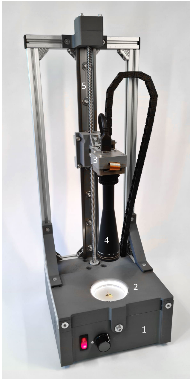
FIGURE 3. The plug-in Entomoscope, with (1) base, (2) lighting, (3) 12 MP Camera with (4) telecentric lens, (5) linear stage.
