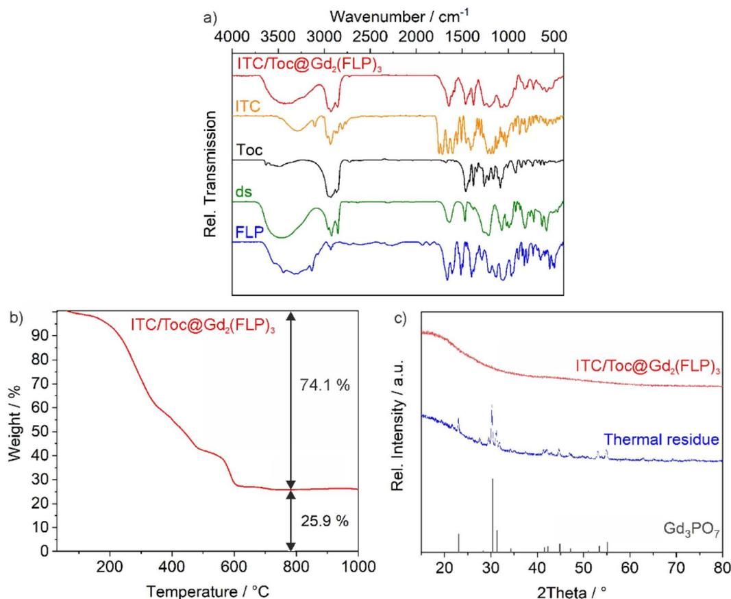
**Fig. 3** Chemical composition of the ITC/Toc@Gd<sub>2</sub>(FLP)<sub>3</sub> nanocarriers: (a) FT-IR spectra with ITC, Toc, SDS and FLP as references; (b) TG analysis; (c) XRD of the as-prepared nanocarriers and of the thermal residue after TG analysis (Gd<sub>3</sub>PO<sub>7</sub>; ICDD-no. 00-034-1066 as a reference).
