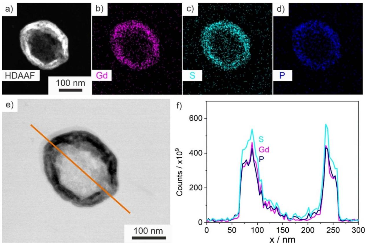
Fig. 6 EDXS of ITC/Toc@Gd<sub>2</sub>(FLP)<sub>3</sub> nanocarriers: (a) HDAAF-STEM image; (b–d) EDXS element mapping for the nanocarriers on (a) with Gd (b), S (c), and P (d); (e) HDAAF-STEM image with EDXS line scan (f) along the orange line for Gd, S, and P.
