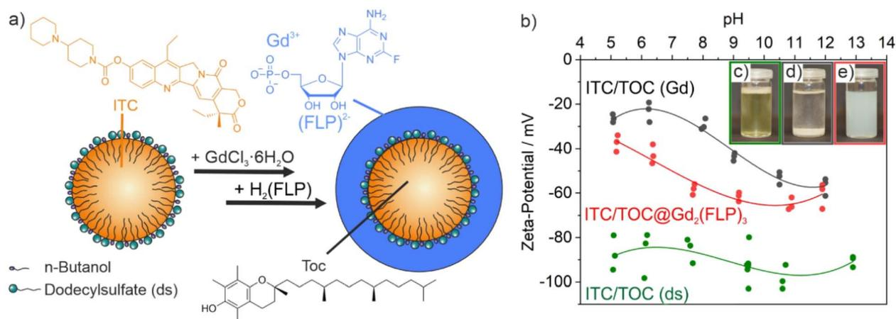
Fig. 1 Synthesis of ITC/Toc@Gd<sub>2</sub>(FLP)<sub>3</sub> nanocarriers: (a) scheme illustrating synthesis conditions and nanocarrier structure; (b) pH-dependent zeta potential over the course of the synthesis with photos of microemulsion with ds-stabilized ITC/Toc (c), colloiddally unstable suspension after addition of Gd<sup>3+</sup> (d), final suspension of ITC/Toc@Gd<sub>2</sub>(FLP)<sub>3</sub> core@shell nanocarriers (e).
