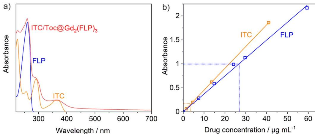
Fig. 4 Photometry of ITC/Toc@Gd<sub>2</sub>(FLP)<sub>3</sub> nanocarriers: (a) UV-vis spectra of ITC/Toc@Gd<sub>2</sub>(FLP)<sub>3</sub> suspension with aqueous solutions of ITC (dissolved in a microemulsion with ds as surfactant) and FLP (in water) as references; (b) UV-vis calibration curves for ITC and FLP (nanocarrier sample diluted by a factor of 12 to fit on the calibration curve).
