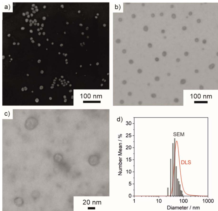
Fig. 5 Size, size distribution, and structure of ITC/Toc@Gd<sub>2</sub>(FLP)<sub>3</sub> core@shell nanocarriers: (a) SEM image, (b and c) STEM images at different levels of magnification, (d) size distribution according to DLS (in water) and according to statistical evaluation of SEM images (>250 particles).
