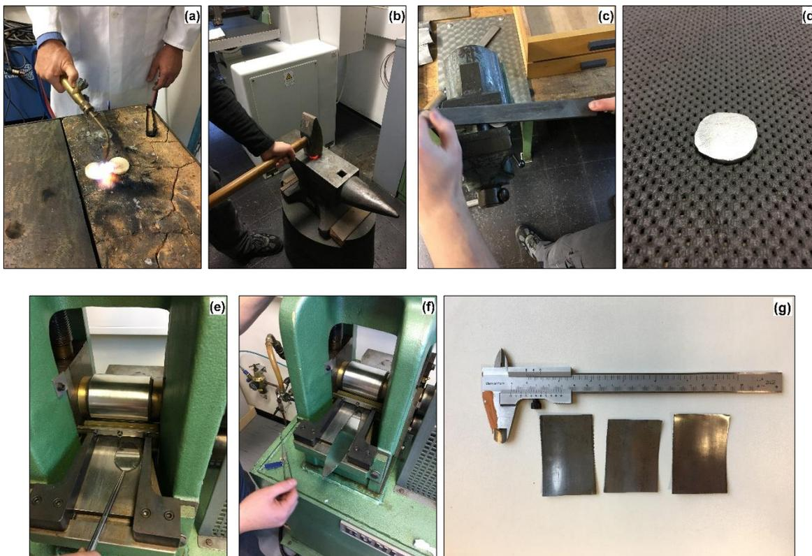
Fig. 11 The production route of sheet from as-cast button: (a) heating of the button with flame, (b) forging of the heated button to make a coin-shape sample, (c) rasping of the forged sample to remove the oxide scales from the surface, (d) the prepared sample for cold rolling, (e) the rolling of the sample, (f) further rolling of the sample to the desired thickness of  $\sim 400 \mu\text{m}$  for this work, (g) the obtained sheets after cutting to smaller parts.
