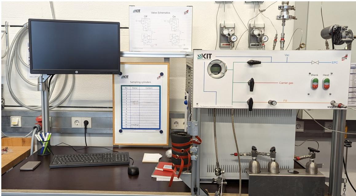
Figure 4.9.: Gas chromatograph bench and valve panel for sample preparation.
