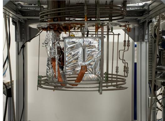
(b) Low-temperature shield covered by multi-layer insulation.
