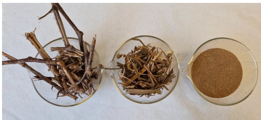
Fig. 1. Gasified biomasses as delivered (left to right: grapevines, Napier Grass, Reed Canary Grass).
