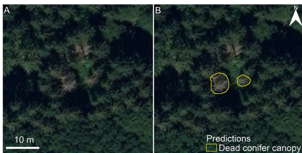
Figure 3. Example of a patch of forest where canopy mortality was not apparent in the reference data but classified correctly by the U-Net. Shown are (A) the aerial image of a forest with few dead tree canopies and some bare forest floor, and (B) the correct detection of the dead tree canopies by the U-Net. The model was able to clearly distinguish between canopy mortality and the bare forest ground.
