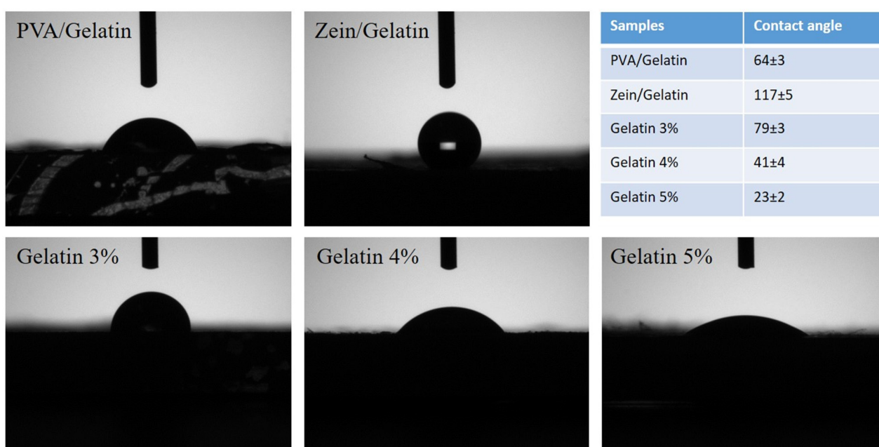
Figure 7. Water contact angle for PVA/Gelatin, Zein/Gelatin, and samples with varying concentration of gelatin.
