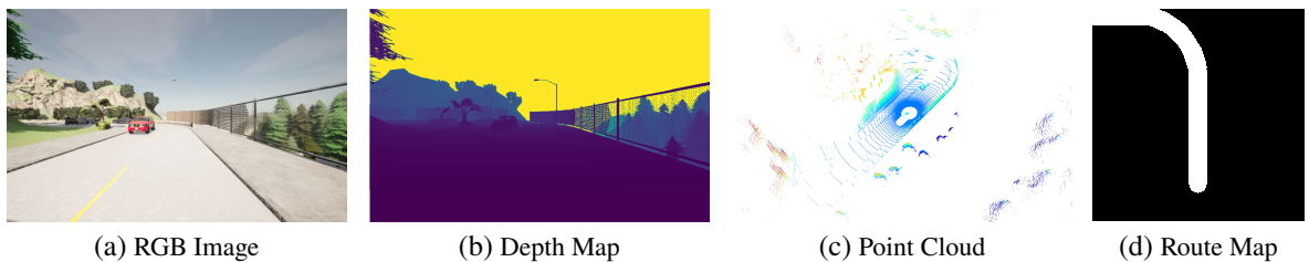
Figure 5.1: Collected data. (a) RGB images and (b) Depth map from the stereo camera; (c) Point cloud from LiDAR, shown in height heat map; (d) Route map shows the planned route in BEV
