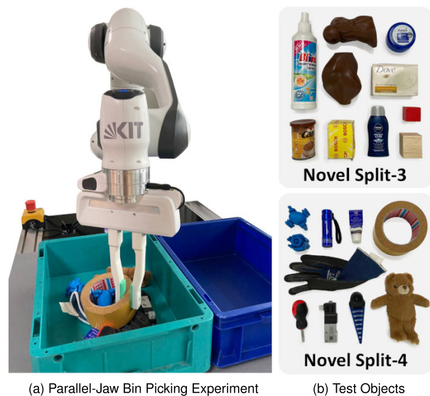
Fig. 16. (a) Robot setup for parallel-jaw grasp experiments. The electrical two-finger parallel gripper (Franka Hand) was customized with enlarged 3D printed fingers to avoid collision with the bin while picking objects close to the wall. (b) Test items are split in two sets: a subset of objects from previous vacuum grasp experiments (split-3) and parallel-jaw only objects (split-4).
