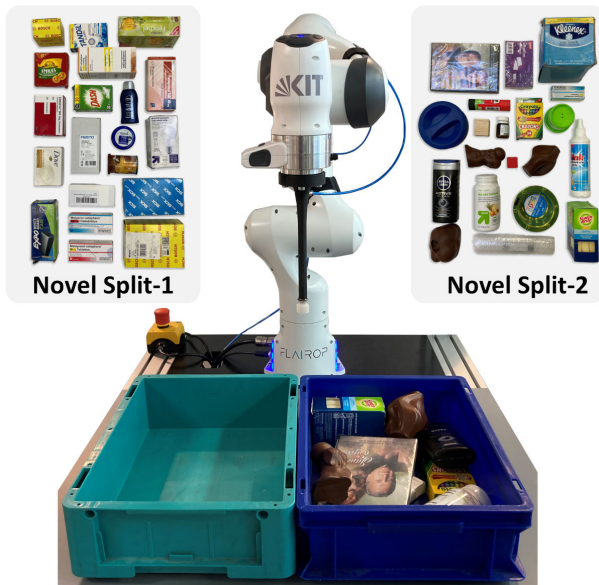
Fig. 12. Physical robot experiments are designed to mimic a real-world logistics use-case, where a robot is tasked with transferring items from one bin to another, as is the case in many order-picking processes. The camera system Zivid Two (not shown) is mounted above the bin, vacuum is generated by an air-powered venturi vacuum pump (Festo VN-07-M-13-PQ2-VQ2-A). The suction cup (Festo ESS-20-CS) has 20 mm diameter. Test objects are divided in two difficulty levels: moderate split-1 and challenging split-2.
