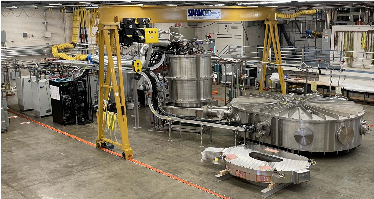
Fig. 3. Photograph of the PSFC Superconducting Magnet Test Facility, as it appeared at the conclusion of TFMC testing in December 2021. The SPARC TFMC appears in the lower-right-hand corner of the photograph.
