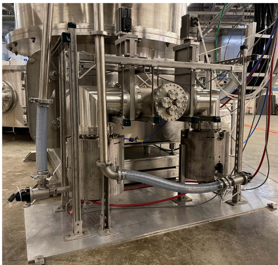
Fig. 8. Photograph of the two turbo pumps and gate valves attached to the back of the current lead cryostat annex.
