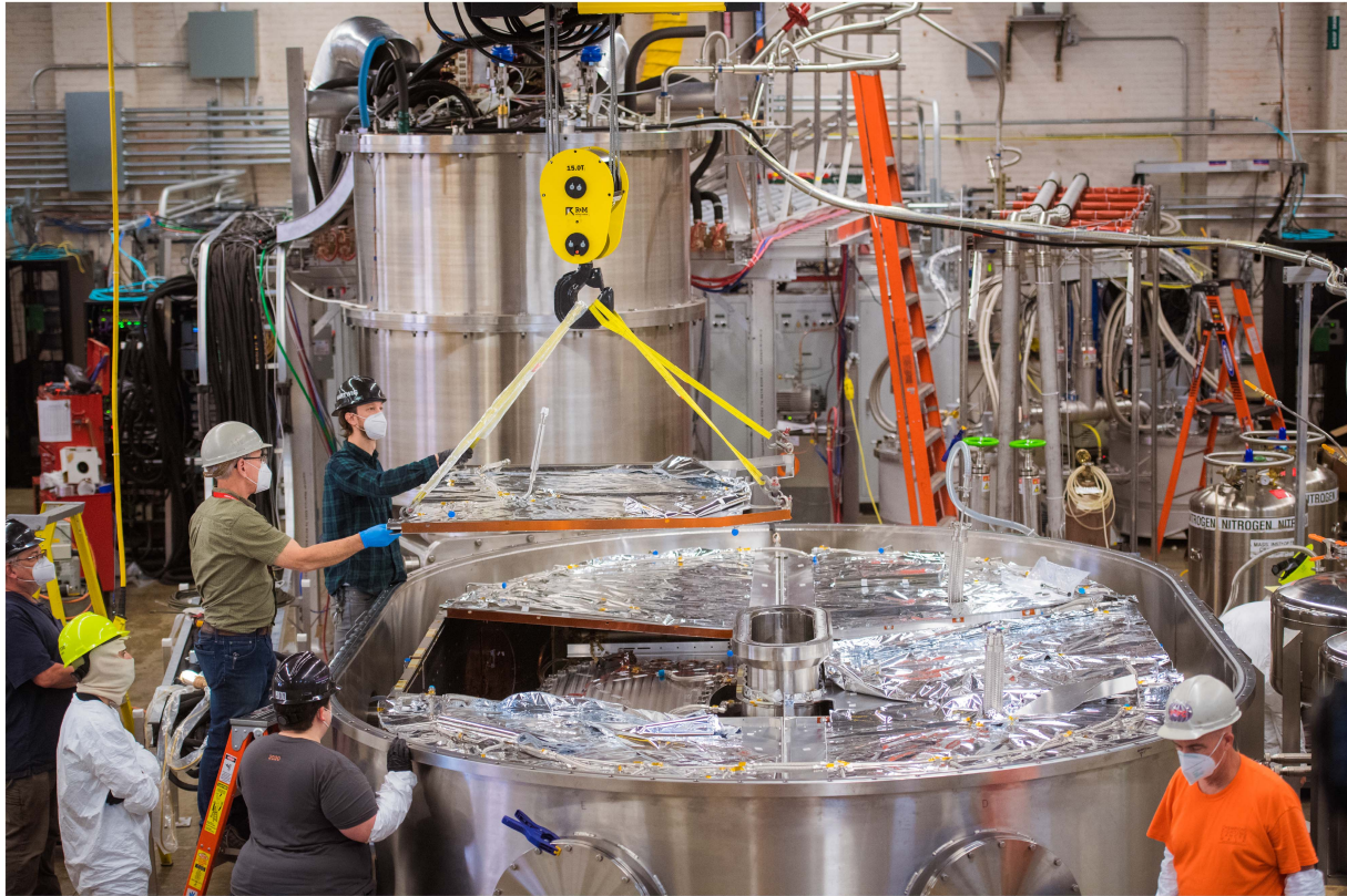
Fig. 7. Installation of the final panel of the main cryostat radiation shield prior to the 20-T campaign. The TFMC is visible underneath. MLI blankets cover the exterior surface of the radiation shield, including ports.
