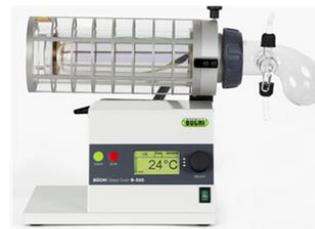
9. Drying of electrodes using BÜCHI Glass Oven B-585
