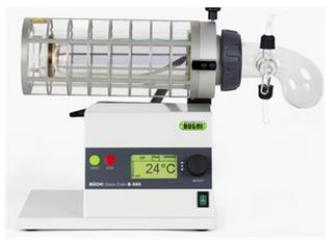
7. Drying of electrodes using BÜCHI Glass Oven B-585
