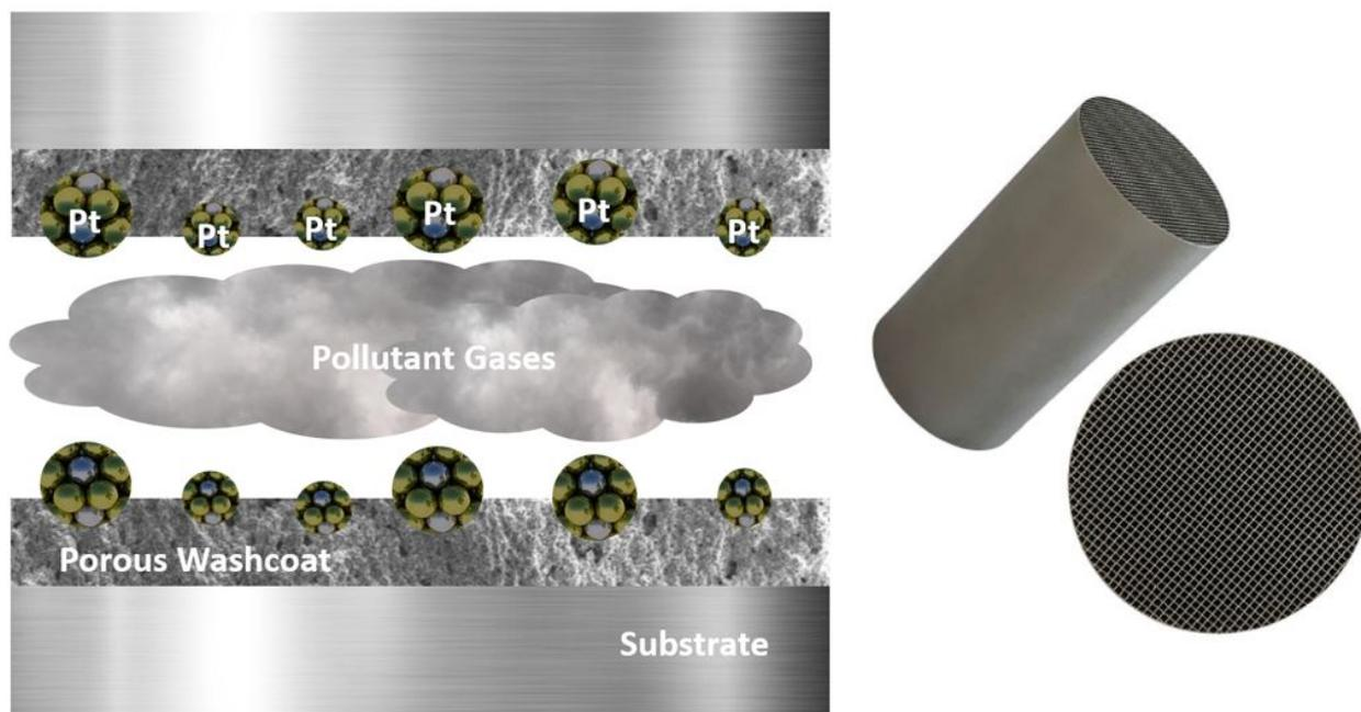
**Figure 1:** Schematic channel cross-section in a supported heterogeneous catalyst. Monolithic substrates are made of metals or ceramics. A porous ceramic layer called washcoat is coated on the top of this substrate to better accommodate the PGMs. Here, Pt nanoparticles in a solid phase are the active species. In this image the size of Pt is exaggerated.
