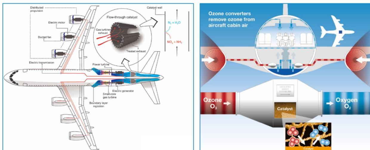
**Figure 4:** Left: Flow-through catalytic converter in hybrid-electric aircrafts (reproduced from Ref. [42] with permission from the Royal Society of Chemistry); Right: Ozone converter [97].
