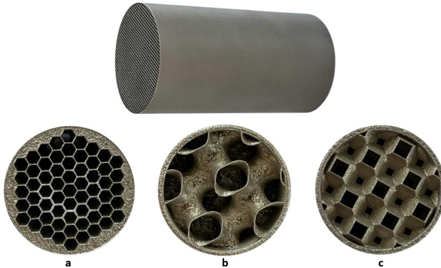
**Figure 3:** Cross-sectional view of the cores of catalytic converters which are additively manufactured via LB-PBF technology: a) Honeycomb-like structure with hexagon channels, b) TPMS structure generated from Gyroid cell with a rotation of  $45^\circ$ , c) Adapted from Schwarz-P cell of TPMS structures and adjusted to the the conditions of a Realizer SLM 125 machine
