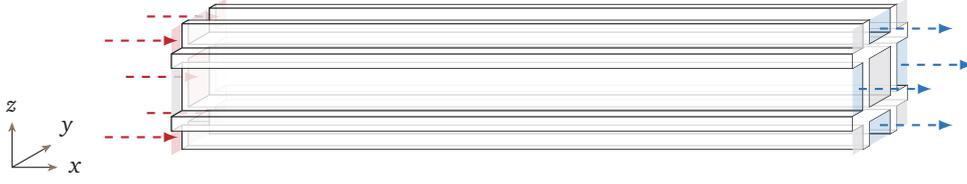
**Figure 5.1:** Sketch of wall-flow filter model, consisting of one central inflow (red) channel with fractions of surrounding inflow and outflow (blue) channels separated by porous walls.
