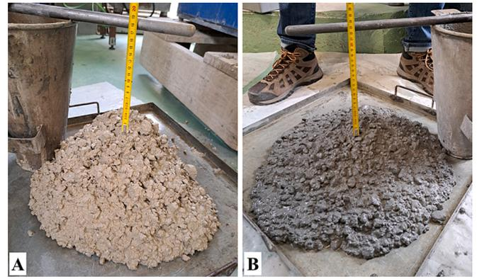
Fig. 3. Slump test (A) OC; (B) HC.
