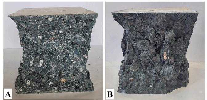
Fig. 4. Typical compressive strength test failure mode (A) OC; (B) HC.
