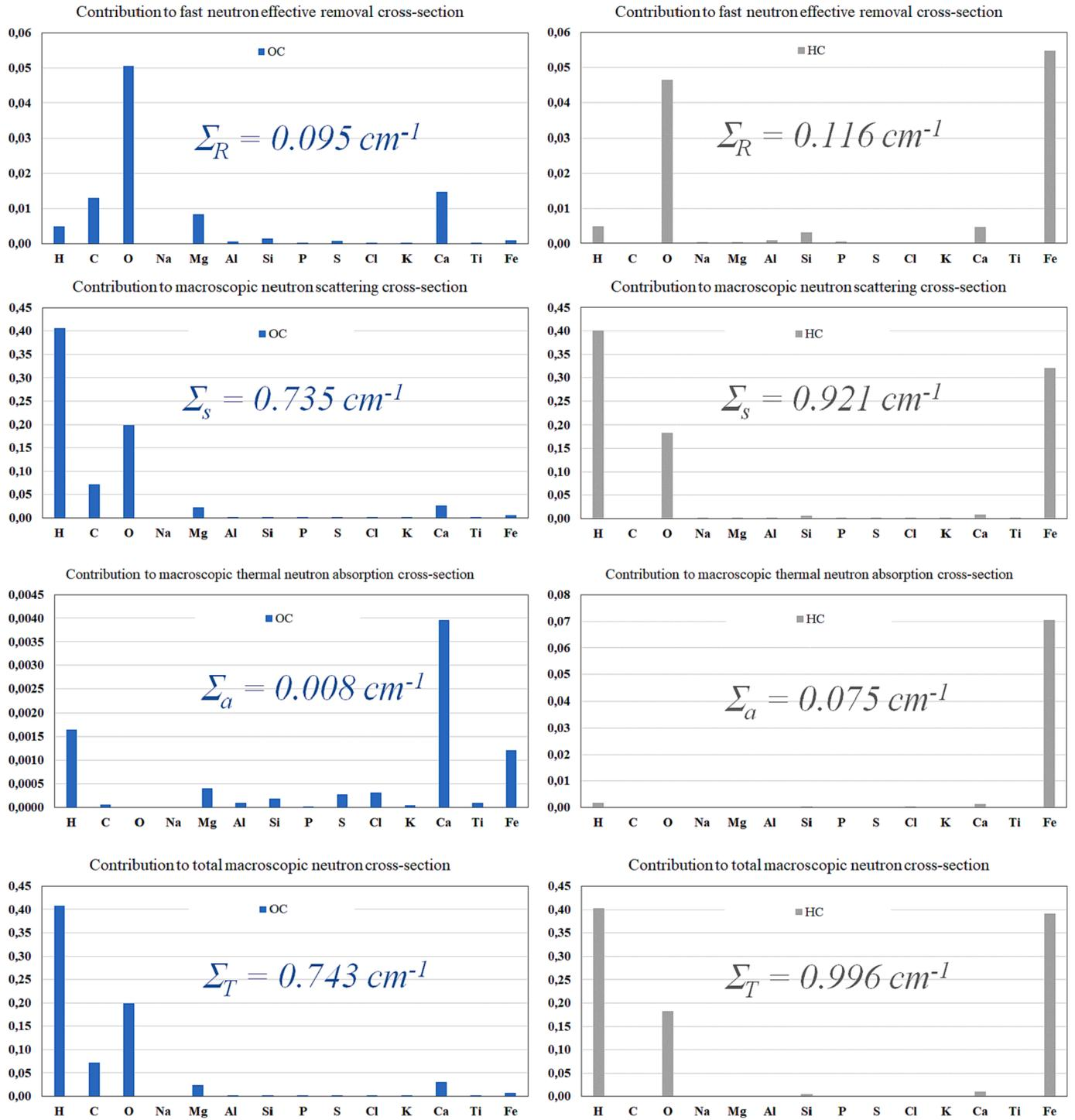
**Fig. 5.** The contribution of each element in concrete and values of neutron shielding efficiency parameters.
