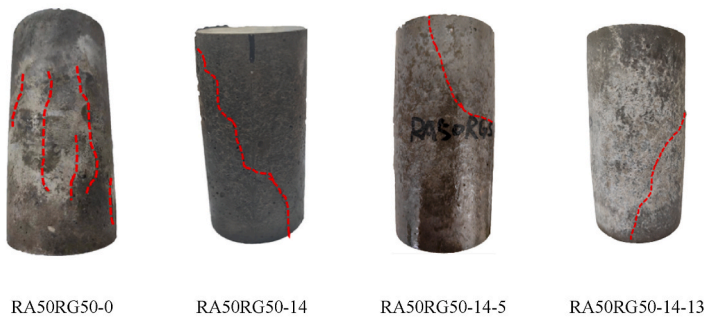
(c) RA50RG50 under different confining pressure and pore water pressure
