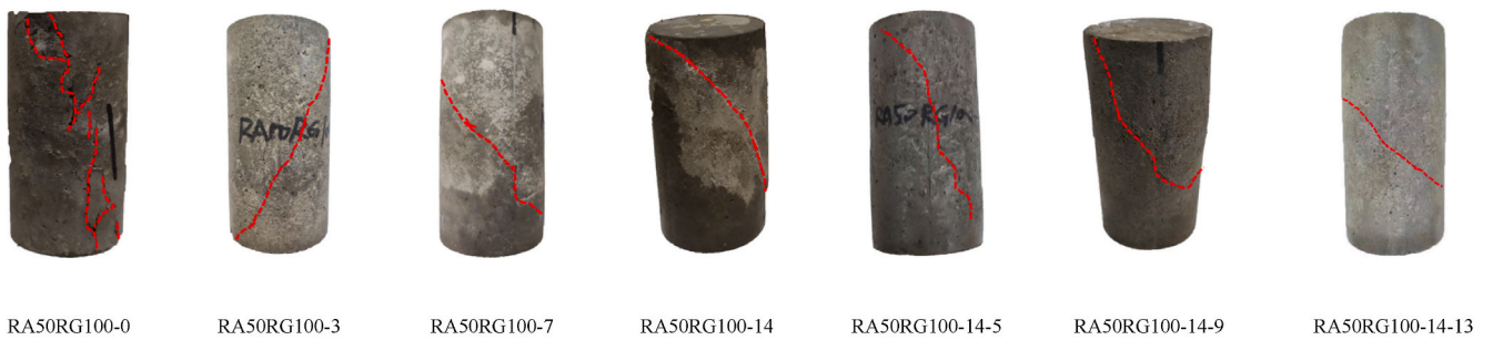
(d) RA50RG100 under different confining pressure and pore water pressure
