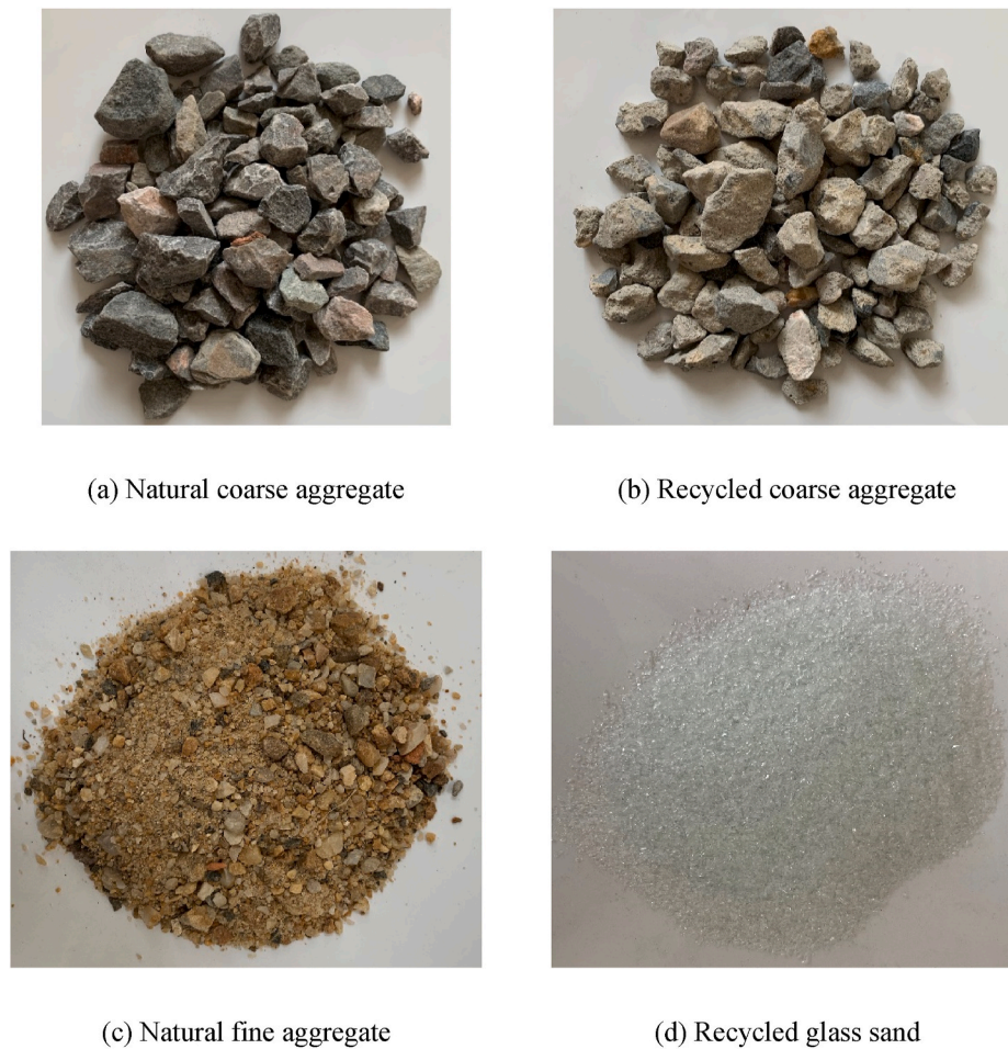
Fig. 1. Coarse and fine aggregate for preparing concrete specimens.
