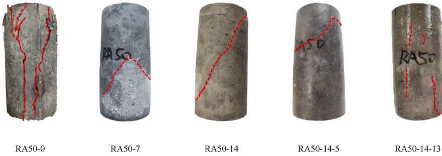
(b) RA50 under different confining pressure and pore water pressure
