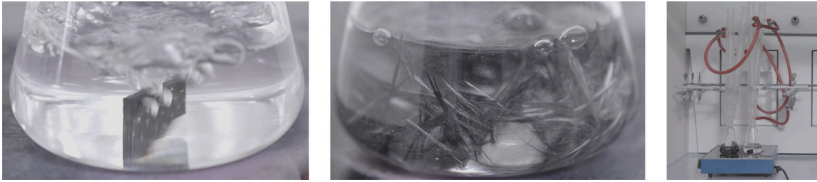
Fig. 3. Drop of a specimen in sulfuric acid in Erlenmeyer flask and dispersion of the fibers. Source: Courtesy of FIBRE Bremen.
