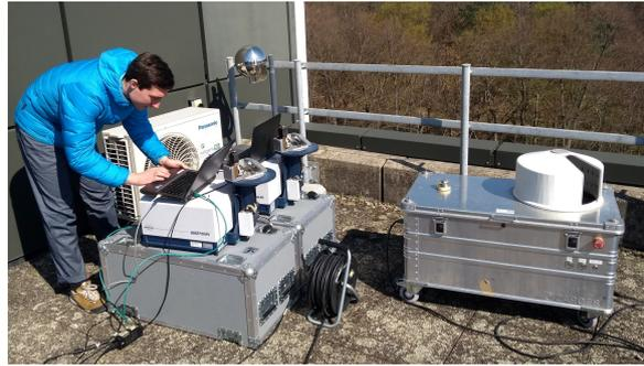
As a second key demand, it is desirable to have comparable ambient conditions when operating the spectrometer at various sites. This helps to avoid systematic errors caused by extreme cold or hot temperatures. Hence, the enclosure should provide a rain cover, a heater, and a cooling mechanism.
