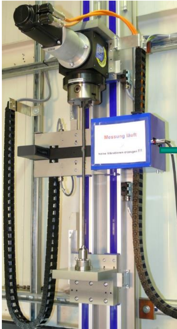
profilometry of clads with laser scanner (thermal expansion ±0.3 μm for ±5 °C)
