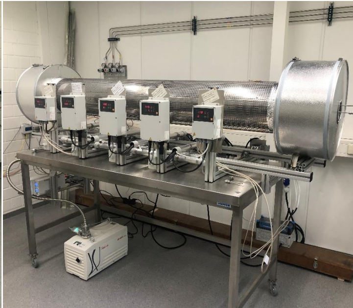
HOKI oven with 5 heated zones and connected gas system
