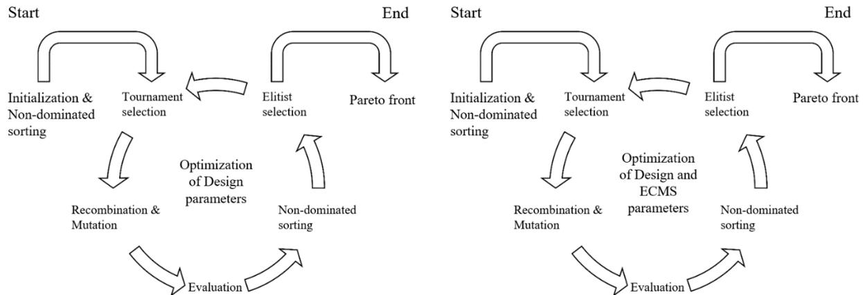
Figure 4: Single-loop optimization approaches A0 (left) and A1 (right)
