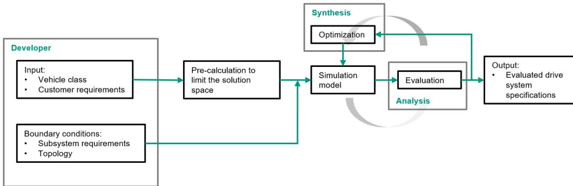
Figure 3: Design approach (schematic) [37]
