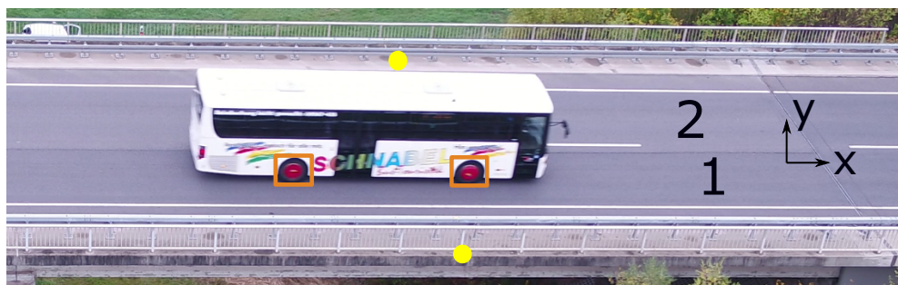
Figure 3. Example of a labeled vehicle using the tool provided by Tzuta [28]. Bounding boxes have been drawn around the axles, as indicated by the orange bounding boxes. The yellow circles represent two control points for the coordination transformation. Furthermore, the lane number is shown.
