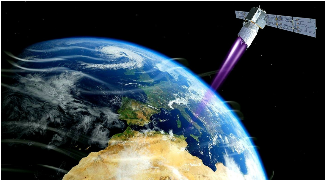
Figure 1.1: The Aeolus satellite measures wind from space using a Doppler Wind Lidar (DWL) called ALADIN. Aeolus emits a laser pulses into the Earth's atmosphere with two different wind detection channels. The Rayleigh channel measures wind from the scattering of air molecules, while the Mie channel captures wind from the backscattering of clouds and aerosol particles, allowing for wind measurements in different atmospheric conditions. Image credit: ESA.
