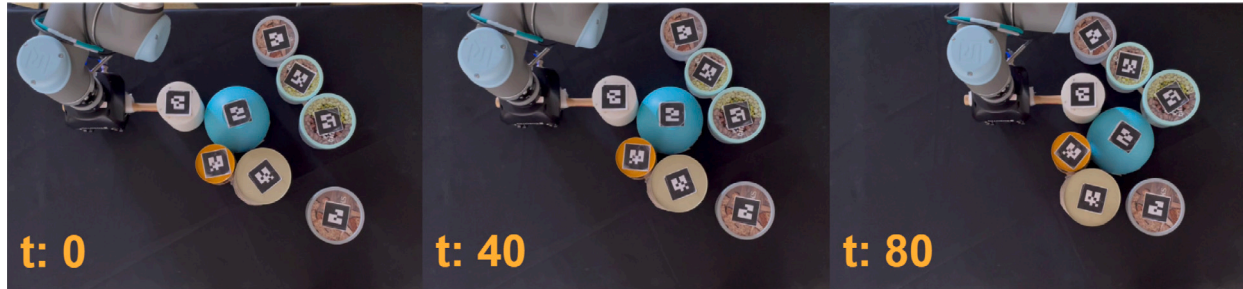
Fig. 16. Snapshots of a robot interaction in a real-world setting. Our framework continuously updates its joint predictions as it observes the motion of objects and predicts their future positions.
