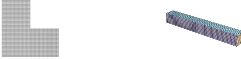
Figure 5.2: Meshes used for MFEM diffusion experiments. Left: L-shape mesh with 7 levels of uniform refinement (49,152 elements); Right: Beam mesh with 3 levels of uniform refinement (4,096 elements).
