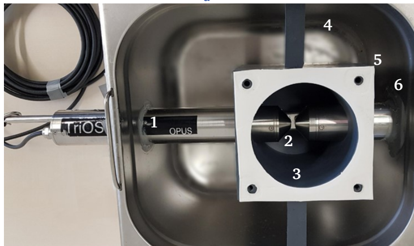
Fig. 5.1: (a) The configuration of the reference system comprises several components, such as an ozone generator (1), medical oxygen (2), sensor processing unit (3), temperature sensor (4), measurement module with a spectroscopic sensor and laboratory water bath (5), and a magnetic stirrer with heating plate (6). [14] (b) Top view of the measurement module, which consists of several components, such as the UV spectroscopic sensor (1), a measurement gap with adjustable light path length (2), the measurement chamber (3), a laboratory water bath (4), a silicone rubber sheet (5), and silicone sealant (6). [14]
