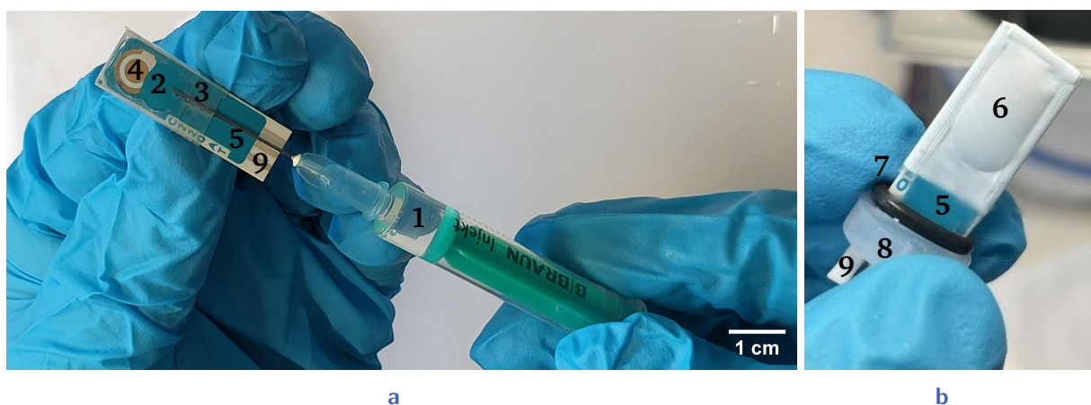
Fig. 9.5: (a) Injecting 0.1 M potassium nitrate electrolyte (1) into the space (2) between PDMS membrane (3) and the active electrode area (4). (Modified according to [351] © 2023 IEEE) (b) Ozone sensor based on commercial screen-printed electrodes (5) with a PTFE membrane (6). The o-ring sealing (7) and silicone sealing (8) are above the conductor paths (9) between the sensor and the potentiostat connection.
