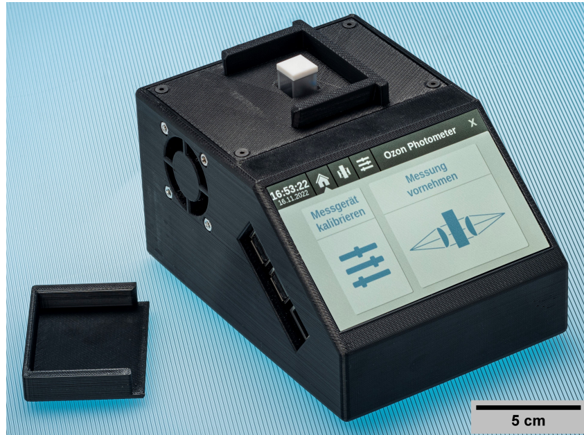
Fig. 8.4: Shows the final photometer configuration with touch-screen; the sliding cover is removed from the photometer's top side. [346] © 2024 IEEE [Image: Markus Breig, KIT]
