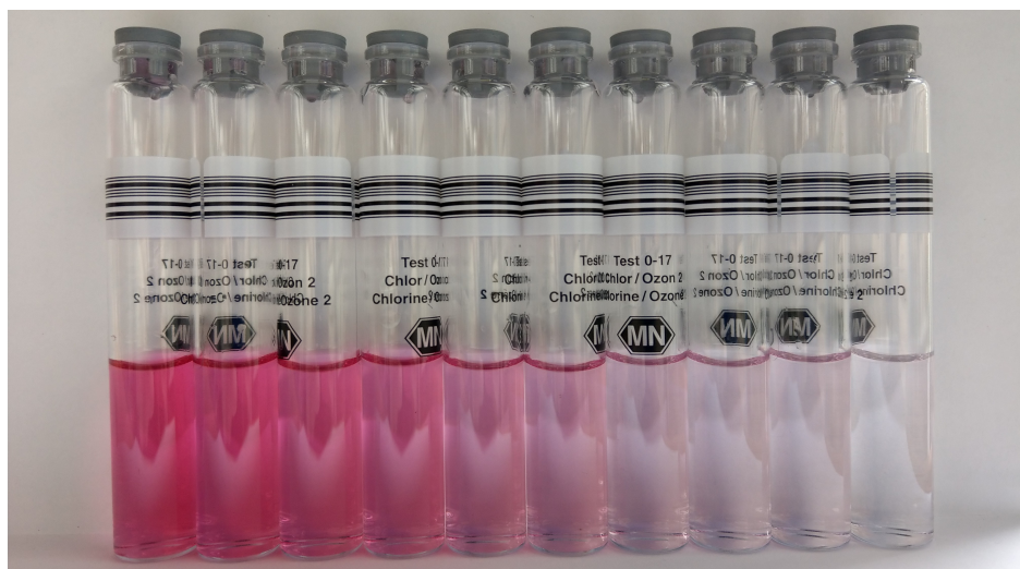
Fig. 3.5: Shows cuvettes with different ozone concentrations and indicator solutions. The darker purple colour of the solution indicates a higher ozone concentration.
