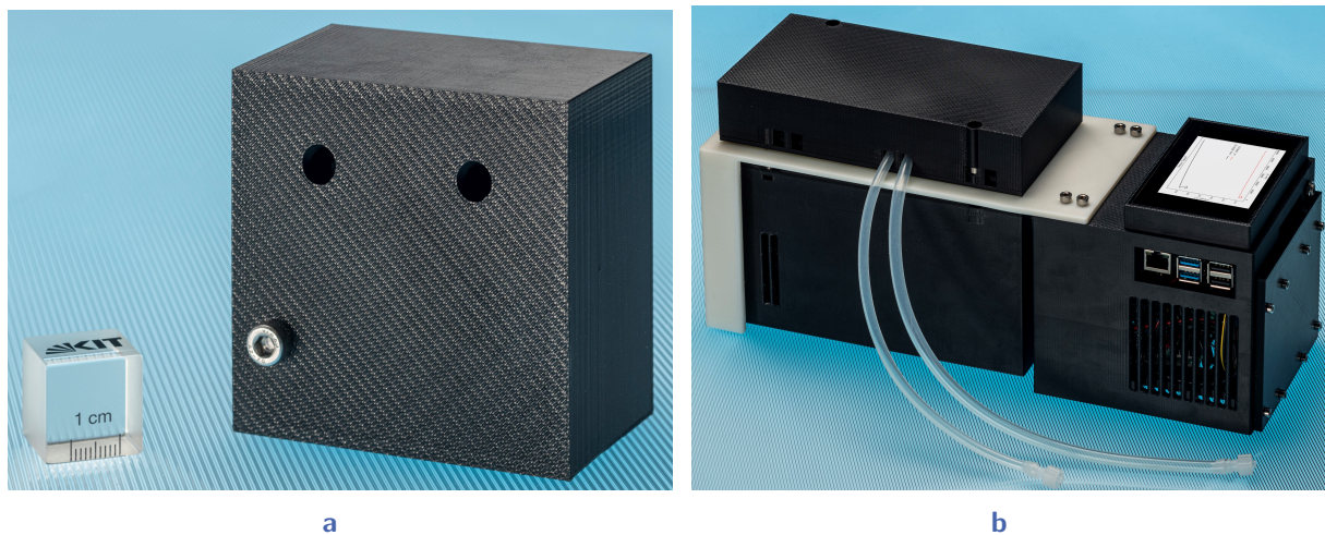
Fig. 7.4: (a) Shows the minimal photometer setup. (b) Depicts the photometer setup with collimating optics. [Images: Markus Breig, KIT]
