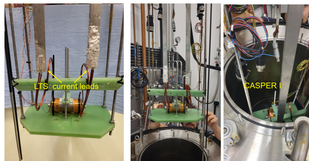
Fig. 11. Measurement setup in CASPER I at liquid helium temperature.
