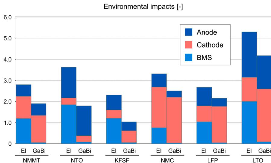
**Fig. 5.** Comparison of the environmental impacts associated with the production of 1 kWh of the six batteries calculated using ecoinvent and GaBi database. The ReCiPe 2016 endpoint method was used for life cycle impact assessment. EI: ecoinvent.
