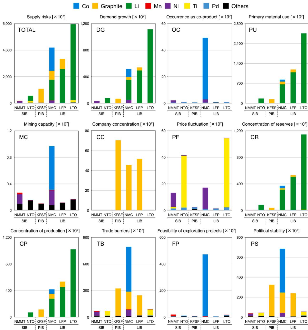
Fig. 4. Contributions of mineral resources to categories of the supply risks for the production of 1 kWh of the six batteries.
