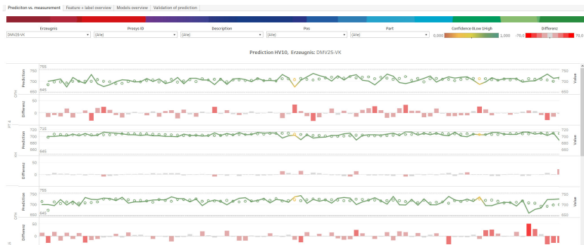
(a) Prediction (circles) vs. measurements (lines) for the solenoid valve
