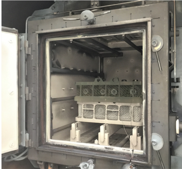
Figure A.5: CH: Picture of IPSEN vacuum furnace used for case hardening nozzle bodies. Black rods are used for heating and white nozzles inject the acetylene
