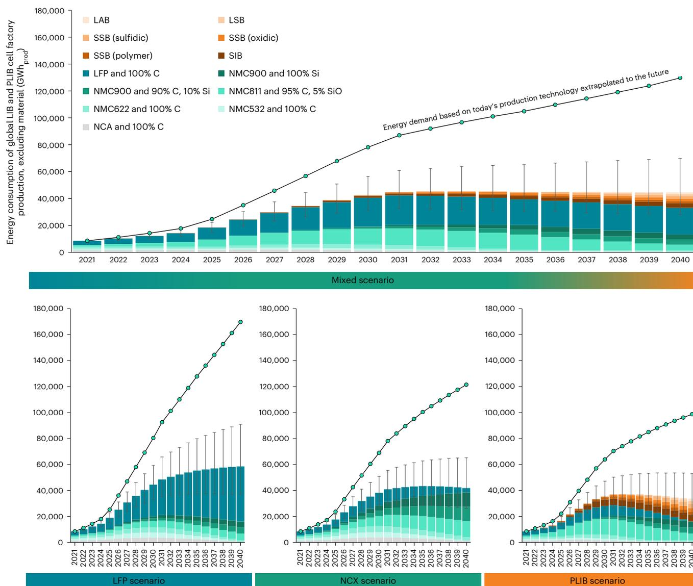
**Fig. 7 | Energy consumption of global LIB and PLIB cell production.** The figure shows the forecast once based on today's technology and know-how level, and once when considering technology improvements, heat pump use and learning effects, as well as economies of scale. This is done for a scenario in which market
