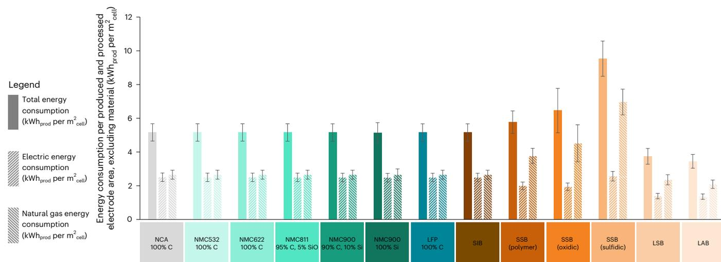
**Fig. 4 | Calculated energy consumption for LIB and PLIB cell production (kWh<sub>prod</sub>) per produced and processed electrode area (m<sup>2</sup><sub>cell</sub>) of a battery cell factory.** Detailed numbers can be found in Source Data Fig. 4. The main bars
