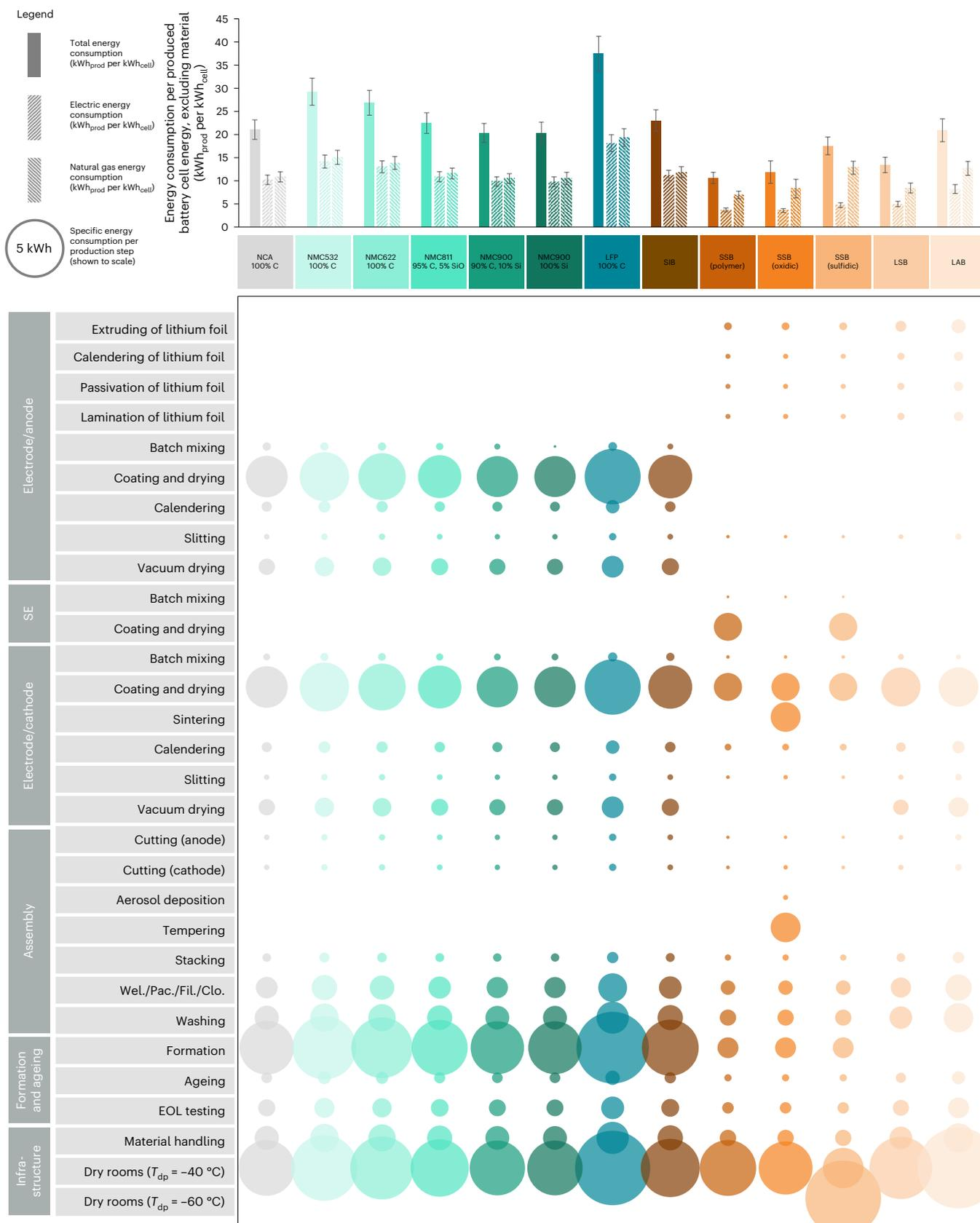
**Fig. 3 | Calculated energy consumption (kWh<sub>prod</sub>) for LIB and PLIB cell production per produced kWh<sub>cell</sub> of cell energy with today's production technology.** The different sizes of the circles represent the different sums of energy (kWh<sub>prod</sub>) of electricity and natural gas. Detailed numbers can be found in Source Data Fig. 3. The main bars show the calculated mean value. The error
