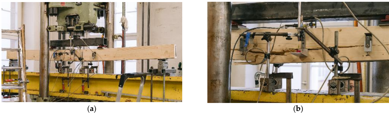
Figure 10. Experimental investigations of specimen V-RS-G-EP2-1. (a) In the testing machine during testing. (b) After failure.
