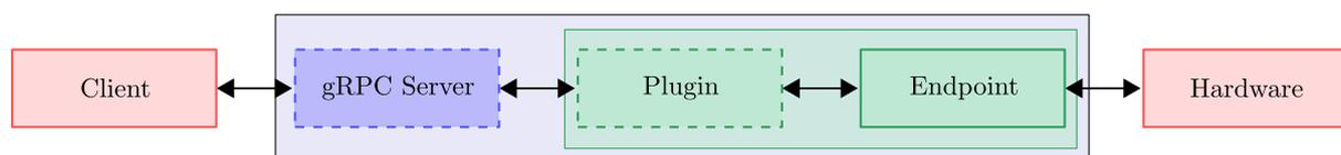
**Figure 4.10:** Sketch of the basic ServiceHub scheme call hierarchy from user to hardware.
