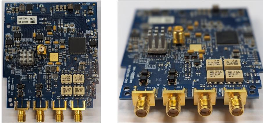
**Figure 4.8:** Selected converter board for prototyping: Analog Devices FMCDQA2 evaluation board.
