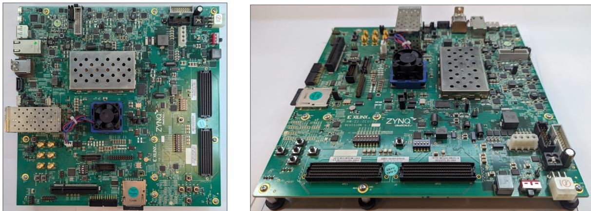
**Figure 4.7:** Selected digital electronics for prototyping, AMD's (ex Xilinx) ZCU102 Evaluation board.
