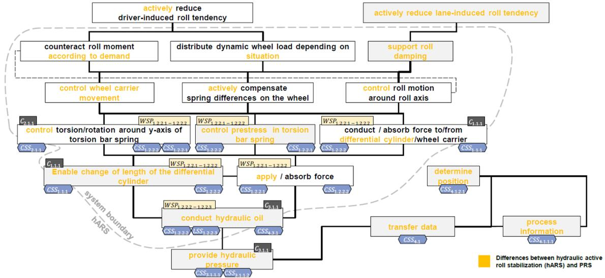
Figure 12: Comparison of the function structure of the hARS and PRS [30]
