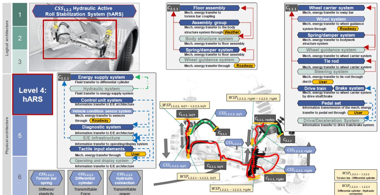
Figure 11: C&C<sup>2</sup> model on level 4: Hydraulic Active Roll Stabilization (hARS) [30]
