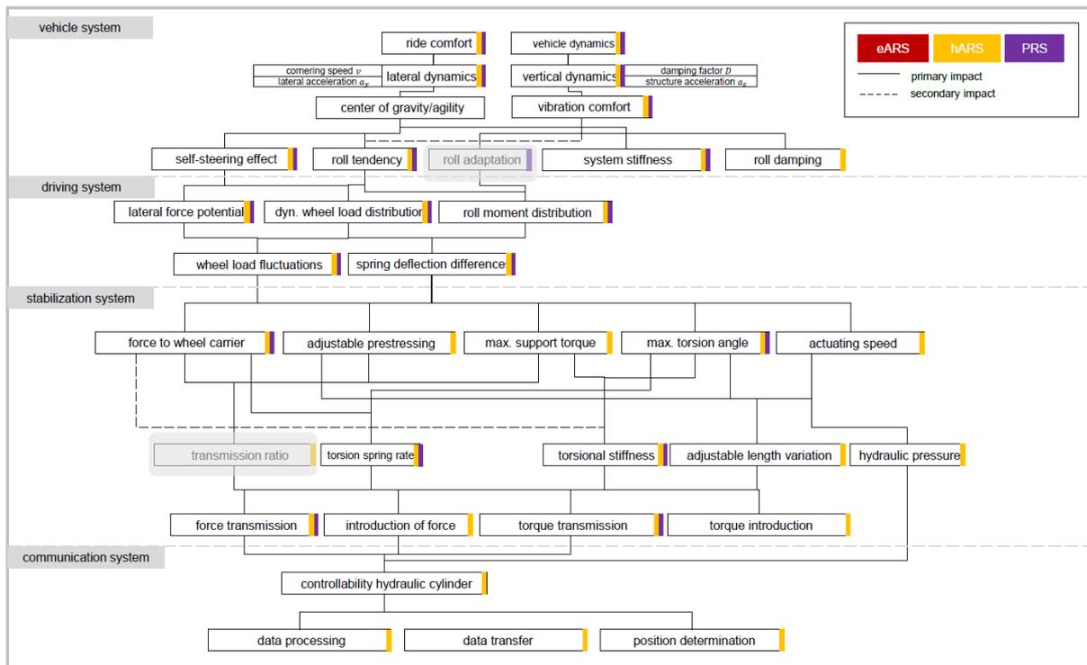
Figure 13: Comparison of the property structure of the hARS and PRS [30]
