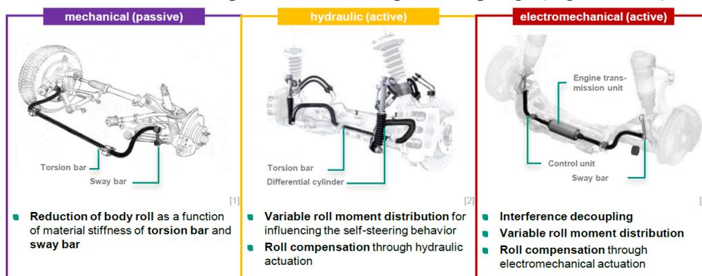
Figure 4: Overview of the alternative reference system elements (RSE) considered for passive, hydraulic active and electromechanical active roll stabilization [30]
