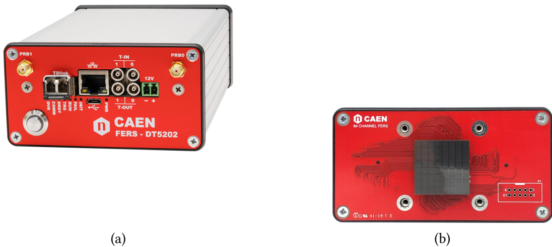
Figure 3.6.: Left: Picture of the DT5202 device from CAEN [42]. Right: Adapter for a Hamamatsu 8x8 SiPM-array [43].
