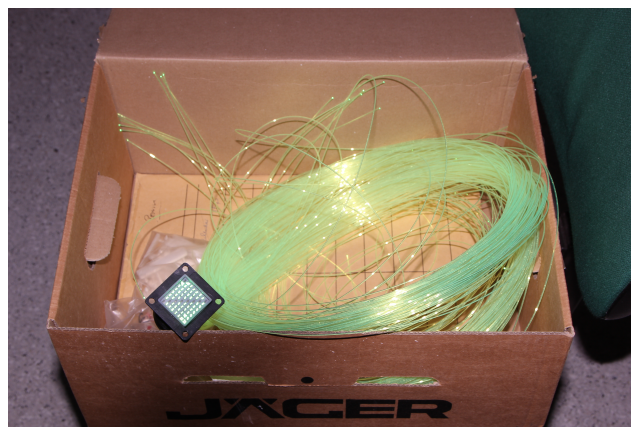
Figure 4.8.: Array mask with fibers securely glued into place. Noticeable are the illuminated fibers, in contrast to the eight non-illuminated fibers along the diagonal and the single non-illuminated fiber in the bottom left corner, as detailed in. With the blank fibers in background.
