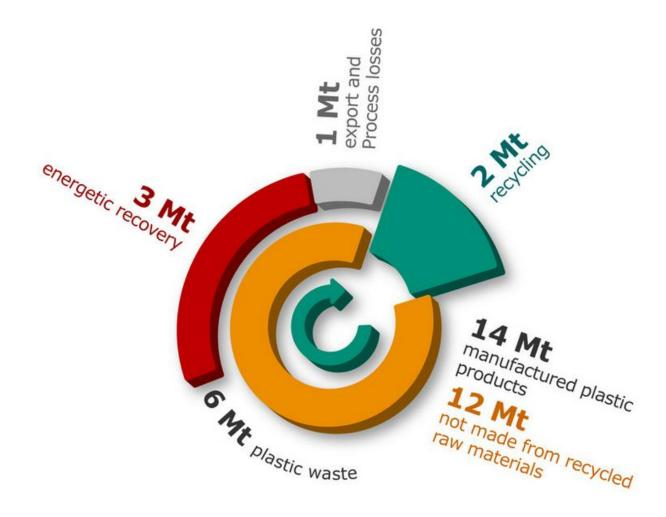
Adapted from the abridged version of the Conversio study www.bkv-gmbh.de Material flow diagram plastics in Germany 2019 published August 2020
