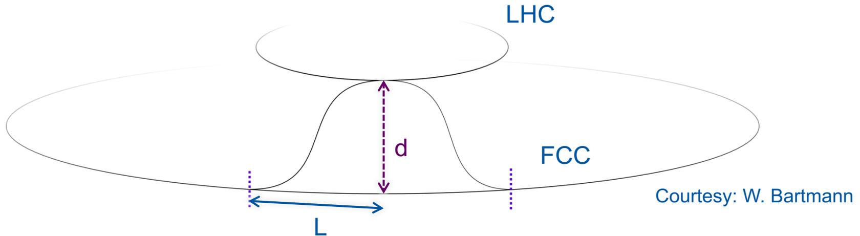
FCC and LHC should overlap, if LHC is used as injector
